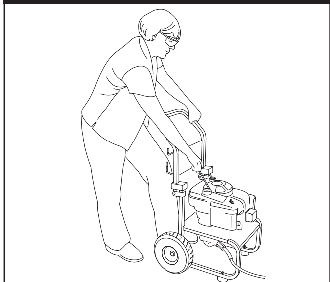
Figure 9 — Recommended Engine Starting Posture
