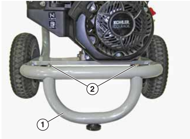
Figure 10 – Installing Front Support
