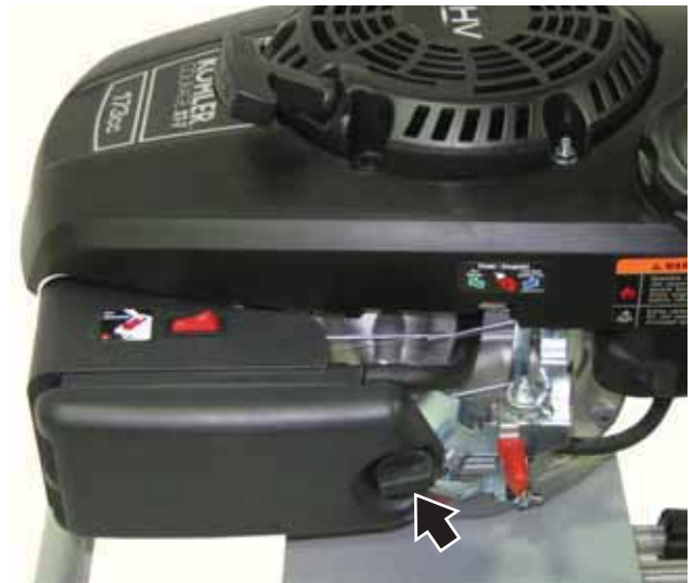
Figure 42 – Opening Air Cleaner Cover
