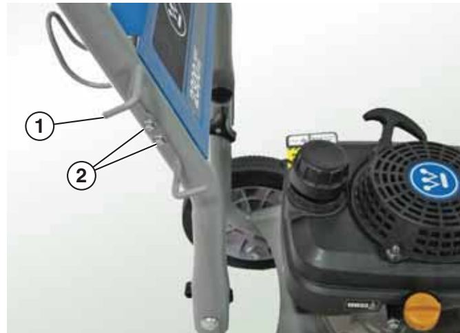
Figure 10 – Installing Spray Gun Bracket
