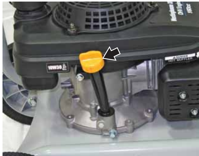
Figure 26 – Oil Fill Plug/Dipstick
