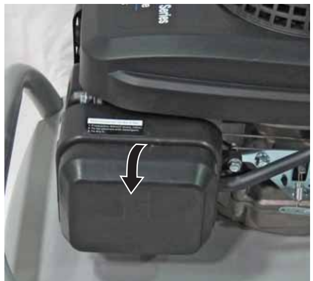
Figure 29 – Removing Air Cleaner Cover
