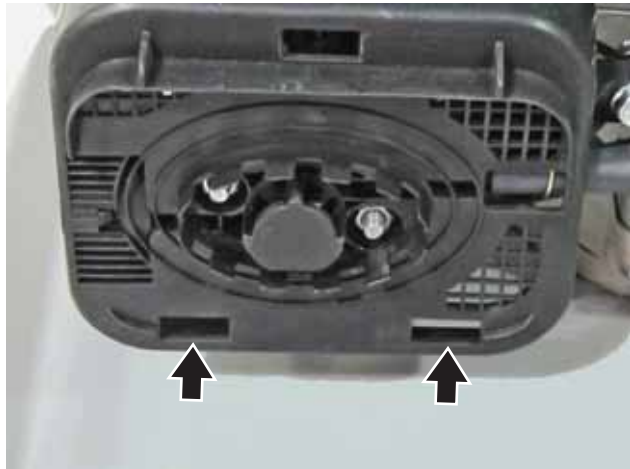
Figure 31 – Installation of Air Cleaner Cover
