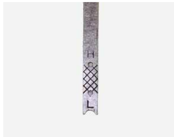
Figure 27 – Checking Oil Level
