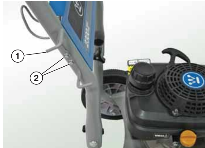
Figure 10 – Installing Spray Gun Bracket
