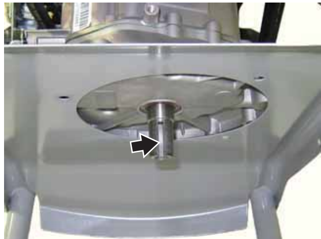
Figure 41 – Key and Crankshaft Keyway
