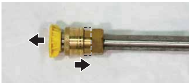
Figure 38 – Spray Tip Removal
