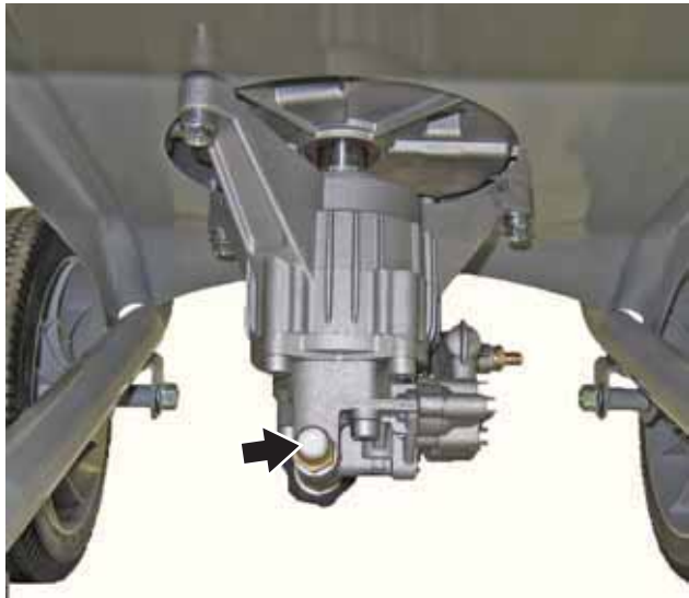
Figure 19 – Pump Thermo Valve
