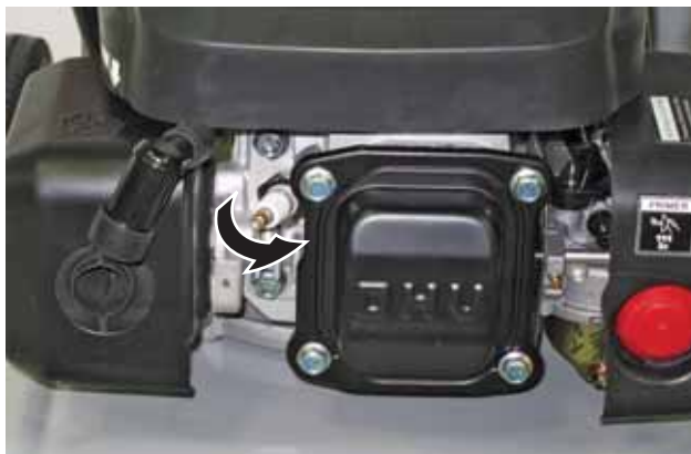
Figure 34 – Removing Spark Plug
