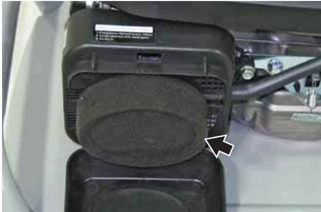
Figure 30 – Removing Air Filter Element
