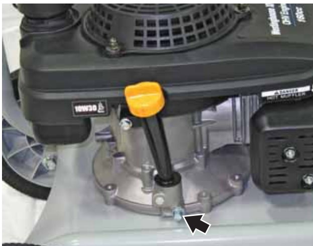
Figure 28 – Oil Drain Plug
