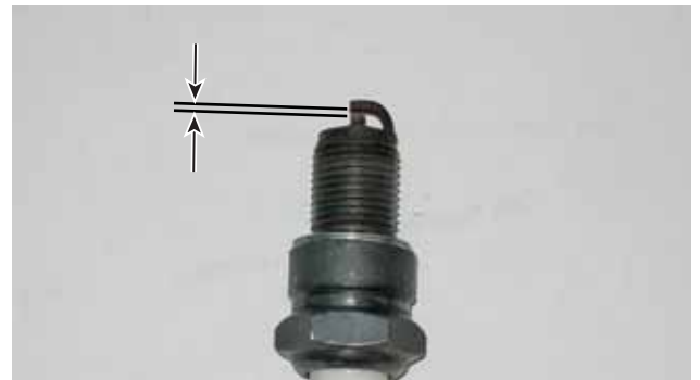
Figure 35 – Spark Plug Gap Requirements
