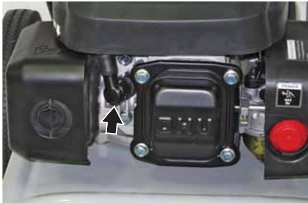
Figure 33 – Removal of Spark Plug Boot
