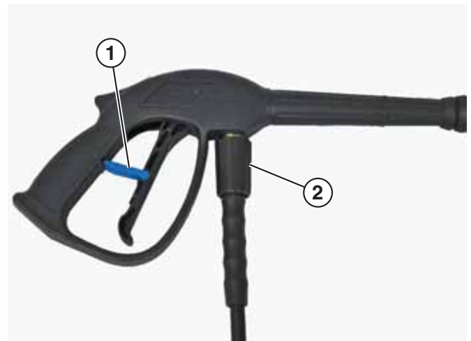
Figure 14 – Trigger Lock in OFF Position
