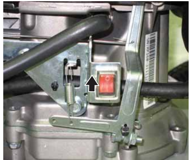
Figure 22 – Engine Stop Switch OFF Position
