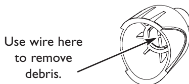
Figure 21 — Nozzle Maintenance
