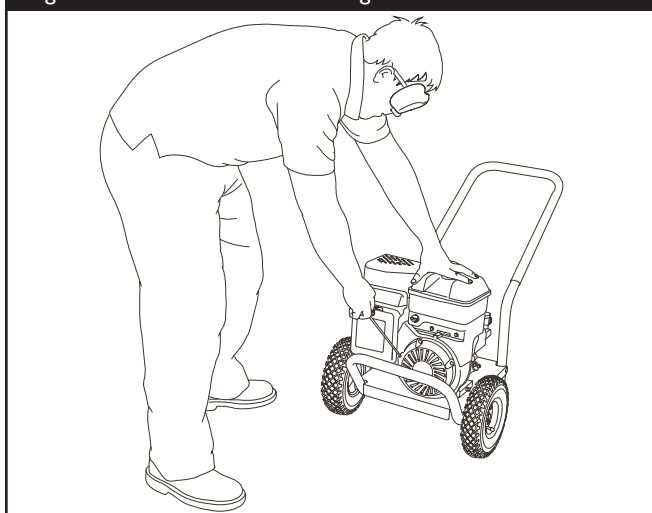
Figure 12 - Recommended Starting Position
