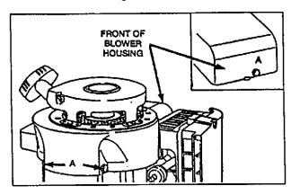
Dirt may clog the engine's air cooling system. The cooling fins and surfaces may require cleaning to prevent overspeeding, overheating and engine damage.
