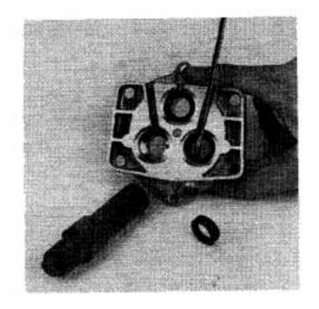
Pass a screwdriver through the leakage grooves and lever out the oil seal rings.
