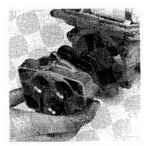
Remove the housing together with the pistons.
