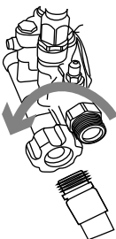
Figure 2-9. Connect Water Supply Hose
