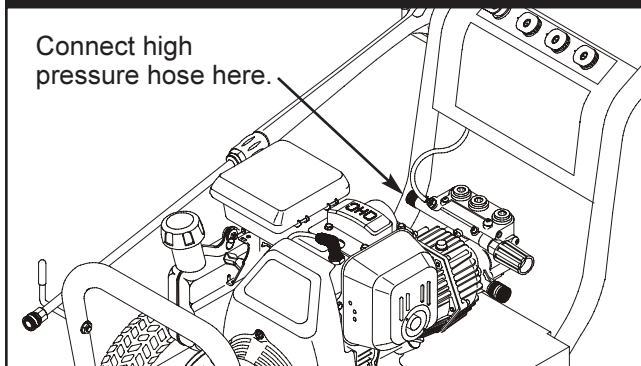
Figure 5 — Connect High Pressure Hose to Pump
