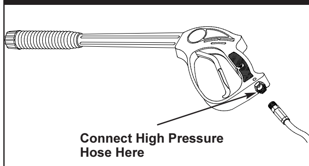
Figure 6 — Connect high pressure hose to spray gun.
