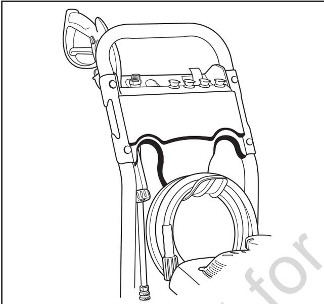
2. Place spray gun through hole on accessory tray on right side of unit.
