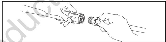
7. Choose spray tip you want to use, pull back on collar of nozzle extension, insert spray tip and release collar. Tug on spray tip to make sure it is securely in place. See *How to Use Spray Tips*.
