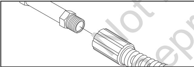
3. Before connecting garden hose to water inlet, inspect inlet screen (A). Clean screen if it contains debris or have it replaced if damaged. DO NOT run pressure washer if inlet screen is damaged.
