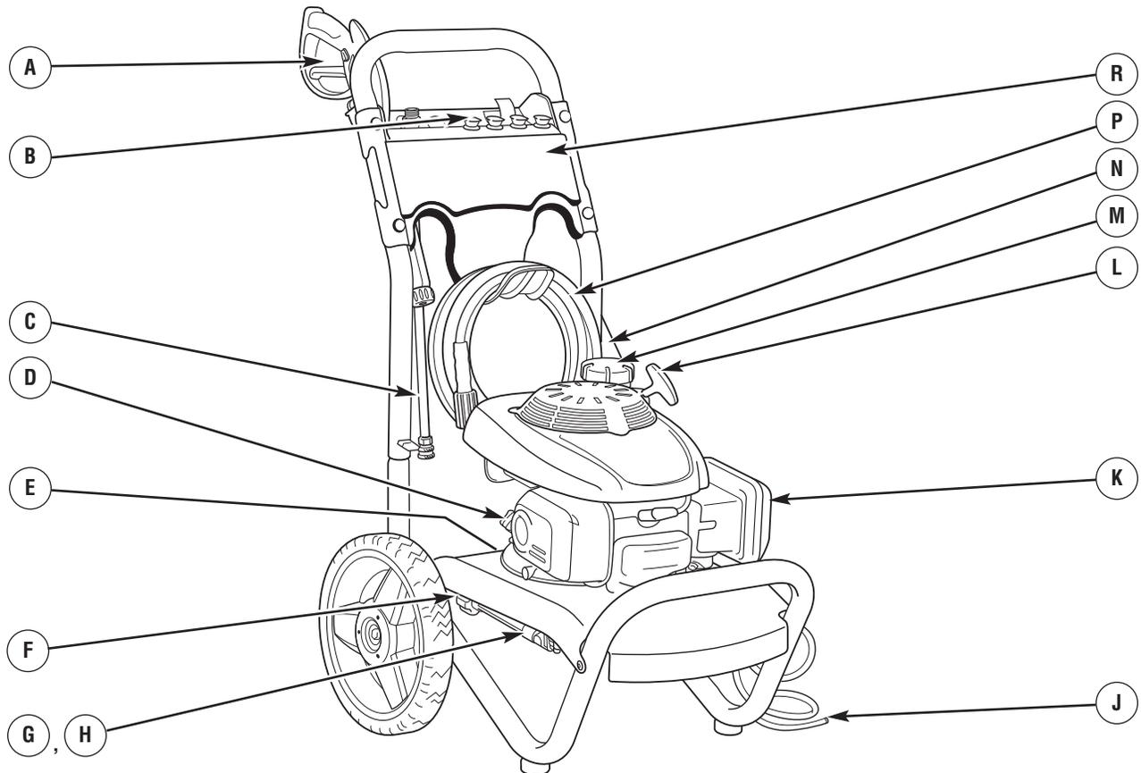
**A - Spray Gun** — Controls the application of water onto cleaning surface with trigger device. Includes trigger lock.
