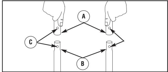
**NOTICE** It may be necessary to move the handle supports from side to side in order to align the handle so it will slide over the handle supports.
