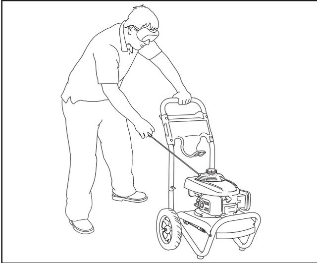
**▲ WARNING** Starter cord kickback (rapid retraction) will pull hand and arm toward engine faster than you can let go which could cause broken bones, fractures, bruises, or sprains resulting in serious injury.
