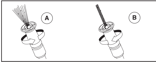
Figure 15: Adjusting the nozzle for spray pattern
