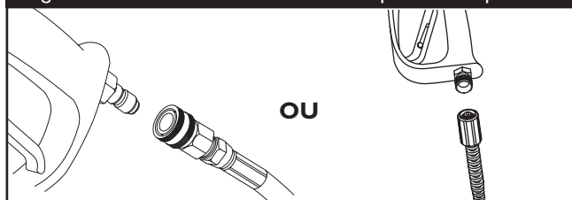
Figure 27 — Raccorder le flexible haute pression au pistolet
