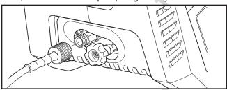
3. Before connecting garden hose to water inlet, inspect inlet screen (A). Clean screen if it contains debris or have it replaced if damaged. DO NOT run pressure washer if inlet screen is damaged.
