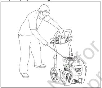
⚠ WARNING Starter cord kickback (rapid) retraction) will pull hand and arm toward engine faster than you can let go which could cause broken bones, fractures, bruises, or sprains resulting in serious injury.
