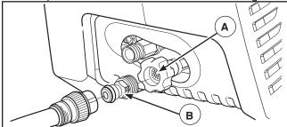
4. Attach garden hose adapter (**B**) to water inlet. Tighten by hand.
