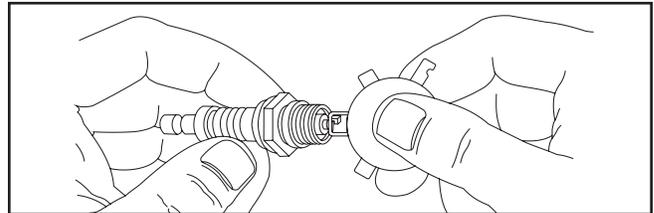
5. Install spark plug and tighten firmly.
