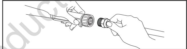
7. Choose spray tip you want to use, pull back on collar of nozzle extension, insert spray tip and release collar. Tug on spray tip to make sure it is securely in place. See *How to Use Spray Tips*.
