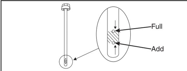
**NOTICE** Pause to permit oil to settle. Wipe dipstick clean each time oil level is checked. DO NOT overfill.
