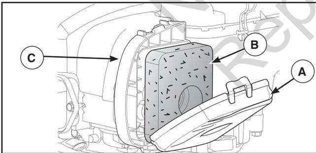
2. Carefully remove air cleaner to prevent debris from falling into carburetor.
