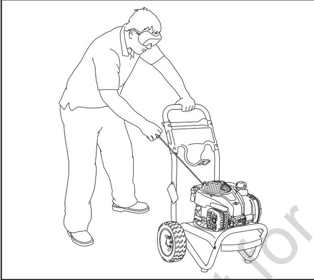
**⚠ WARNING** Starter cord kickback (rapid retraction) will pull hand and arm toward engine faster than you can let go which could cause broken bones, fractures, bruises, or sprains resulting in serious injury.
