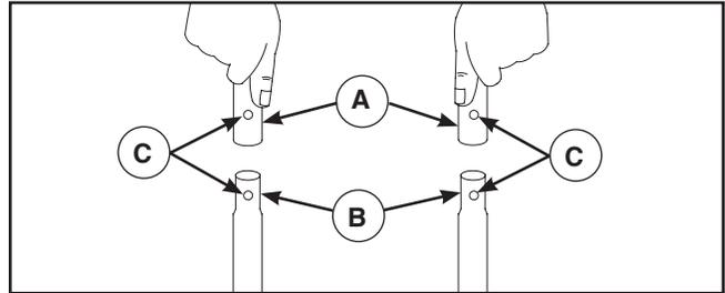
**NOTICE** It may be necessary to move the handle supports from side to side in order to align the handle so it will slide over the handle supports.
