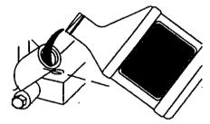
Install oil fill cap, hand tighten securely.
