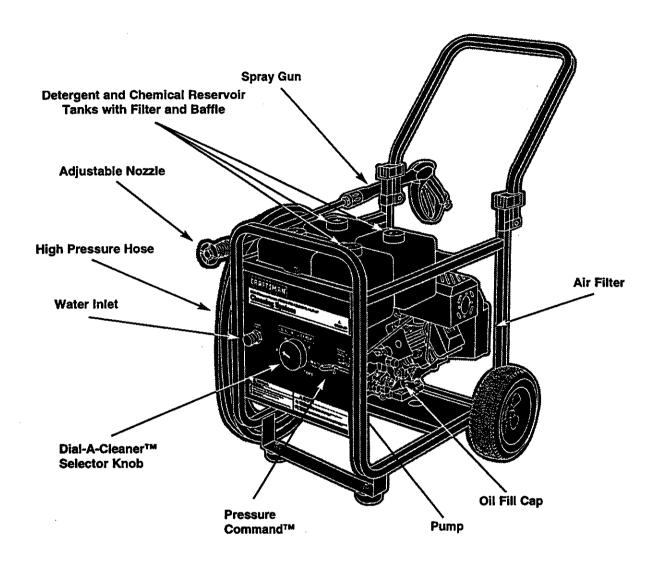
Adjustable Nozzle – Adjust for high or low pressure; narrow or fan spray.
