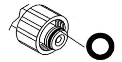
2 O-rings, yellow, (p/n B2264) for the ends of the high pressure hose.
