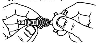
Install spark plug, tighten securely.
