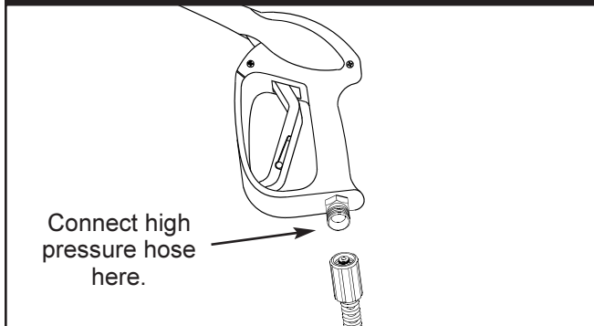
Figure 5 — Connect High Pressure Hose to Spray Gun
