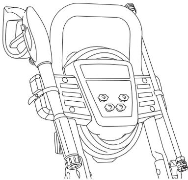
3. Place spray gun in groove on accessory tray as shown. Pull rubber strap tight around spray gun and place hole in strap over tab on accessory tray.
