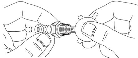
5. Install spark plug and tighten firmly.
