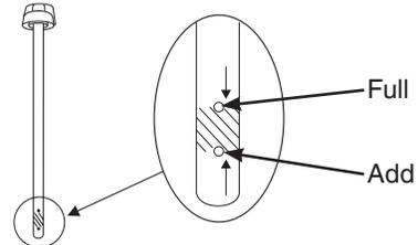
**NOTICE** Pause to permit oil to settle. Wipe dipstick clean each time oil level is checked. DO NOT overfill.
