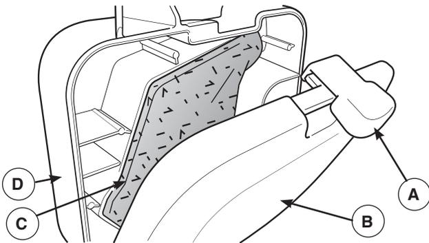
2. Carefully remove air cleaner to prevent debris from falling into carburetor.
