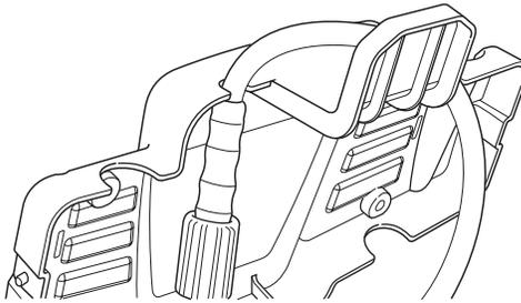
2. Place nozzle extension in groove on accessory tray as shown. Pull rubber strap tight around nozzle extension and place hole in strap over tab on accessory tray.
