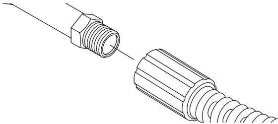
3. Before connecting garden hose to water inlet, inspect inlet screen (A). Clean screen if it contains debris or have it replaced if damaged. **DO NOT run pressure washer if inlet screen is damaged or missing.**
