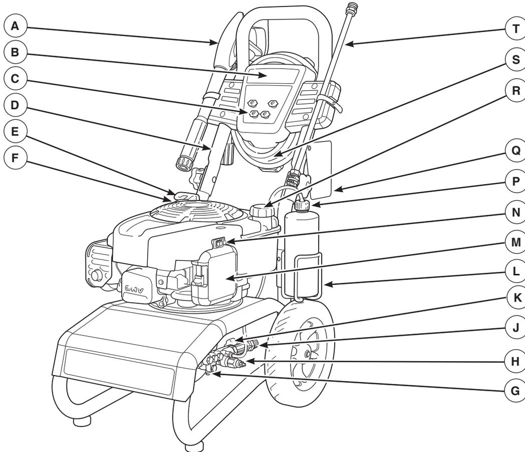
**A - Spray Gun** — Controls the application of water onto cleaning surface with trigger device. Includes trigger lock.
