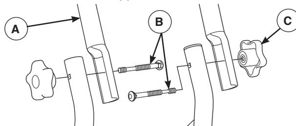
2. Insert handle carriage bolts (B) through holes from inside of unit and attach a plastic knob (C) from outside of unit. Tighten by hand.
