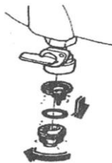
Fuel Filter Element Removal
