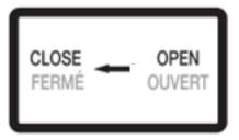
When cold-starting, close the choke. When warm-starting, open the choke.
