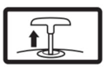
When starting engine, pull cord slowly until resistance is felt then pull rapidly to avoid kickback.
