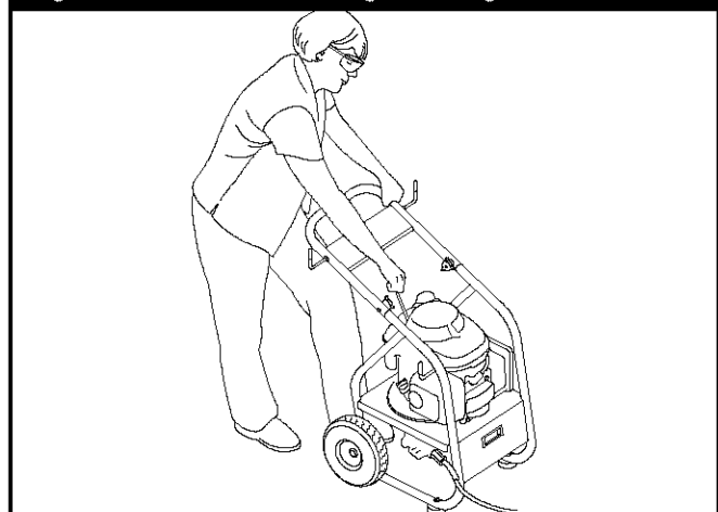
Figure 14 — Recommended Engine Starting Posture
