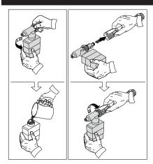
The use of detergents can dramatically reduce cleaning time and assist in the removal of difficult stains. Some detergents have been customized for pressure washer use on specific cleaning tasks. These detergents are approximately as thick as water. The use of thicker detergents, such as dish soap, will clog the chemical injection system and prevent the application of the detergent.
